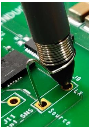
Figure 3-2: Recommended HV probe connection for observing Drain-Source voltage (Left image). Voltage probe with Spring Type Ground lead identified (Right image).
